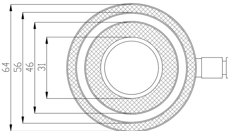
Figure 1. The gripping surface and magnetic poles of MAP-30.
