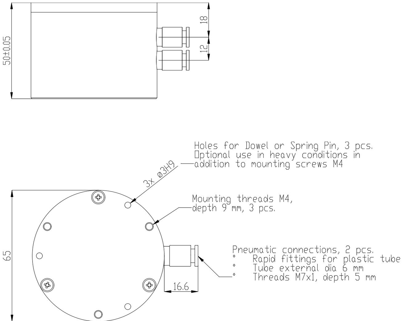
Figure 4. Mounting dimensions of MAP-30.
