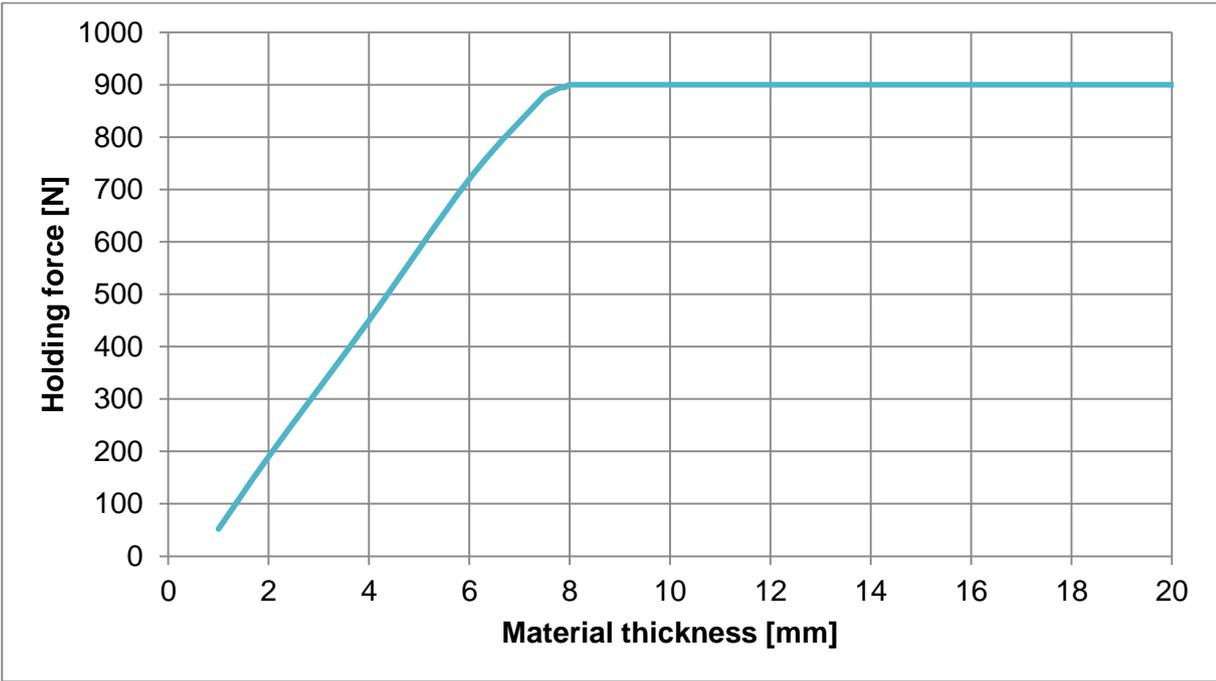
Figure 2. MAP-30 holding force in proportion to material thickness
